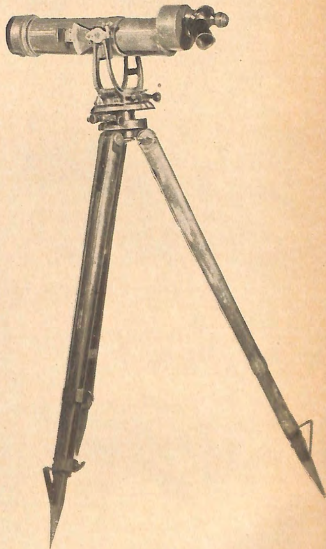
Figure 301. This artillery spotting telescope may be used with three different eyepieces, each of which gives a different magnification—the maximum being 33 power. Provision is made to measure azimuth, and elevation (from -30^{\circ} to +30^{\circ} ).
